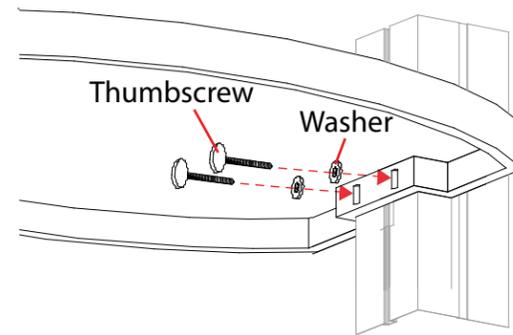
After setting counter on horizontal support, put washer on thumbscrew, and attach thumbscrew through counter to vertical extrusion as shown.
