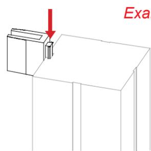
Slide connector on back of A10 clamp into groove of extrusion.
