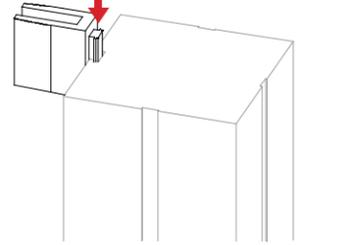
Slide connector on back of A10 clamp into groove of extrusion.
