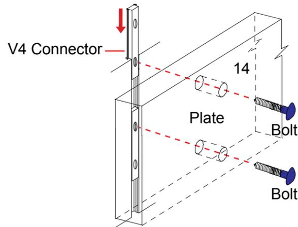
Slide V4 connector into groove of vertical extrusion. Tighten set screw to secure V4 connector in place at correct elevation. Bolt through hole of horizontal plate into threaded hole of V4 connector. Twist and tighten bolt to secure in place.
