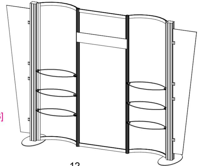
**\*\*Note: Keep vertical extrusions [2 & 8] and [9 & 3] assembled when shipping.**
