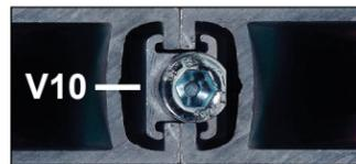
Slide V10 pressure screw between grooves of extrusions. Tighten setscrew to secure pressure in place.
