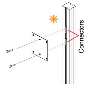
Attach monitor mount back plate to connectors using setscrews provided.
