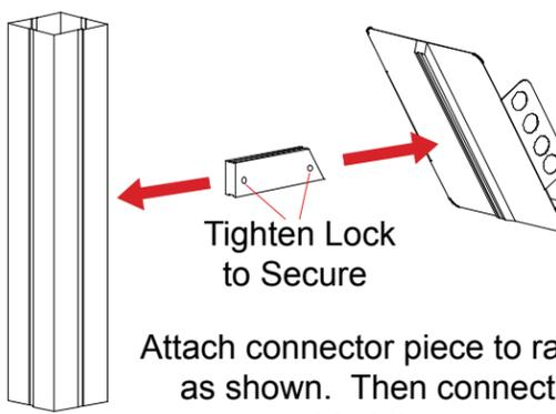
Tighten Lock to Secure
